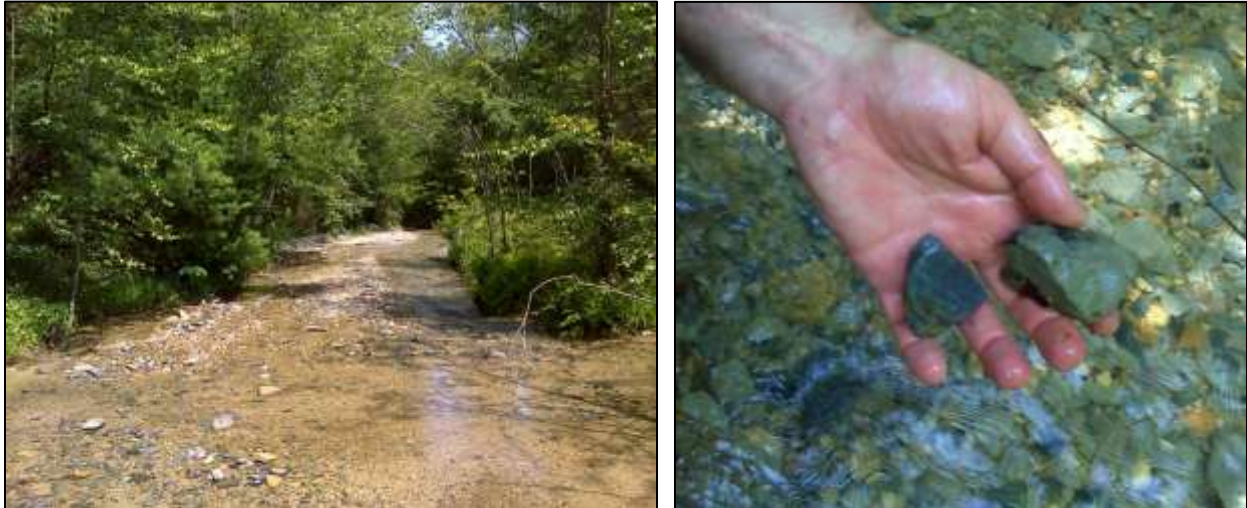
Photos 1 and 2. View of Big Creek where limestone was previously installed (left). View of uncoated and coated limestone rocks in the Big Creek headwaters area (right).
