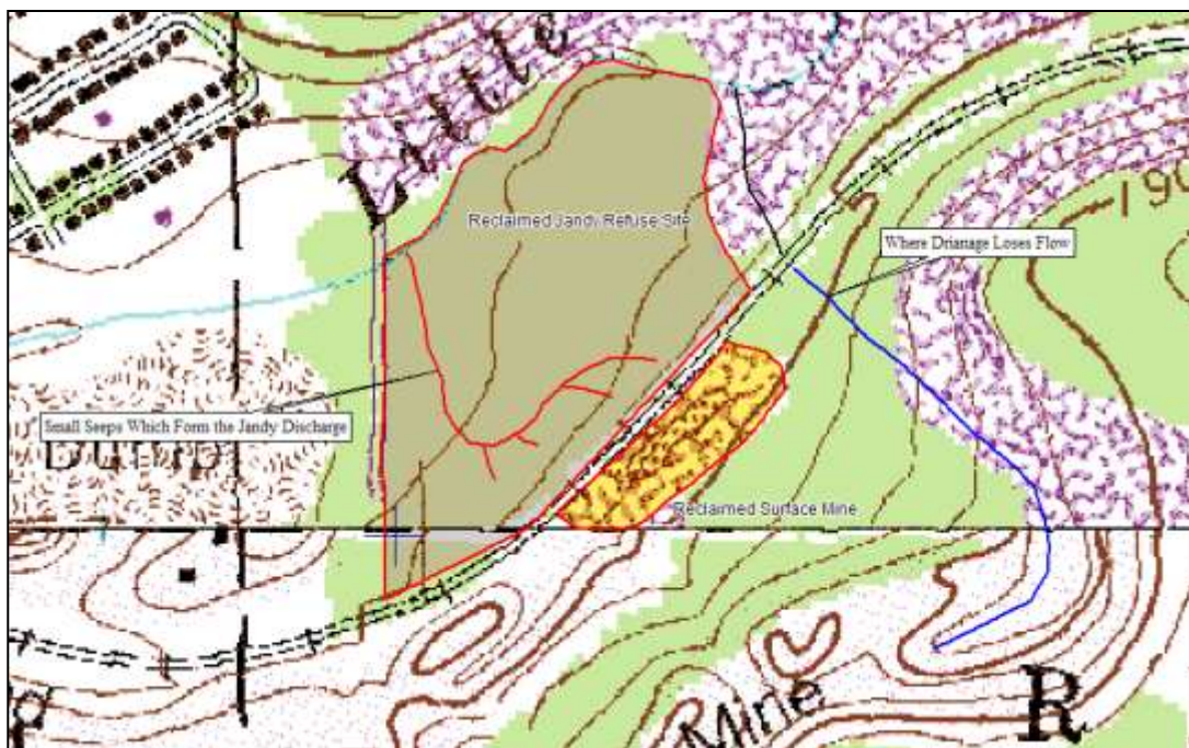
Figure 18. Drainage pattern of Jandy Discharge
