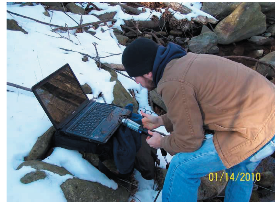
Researcher Scott Collenberg shown downloading data from a HOBOT logger to his laptop.
