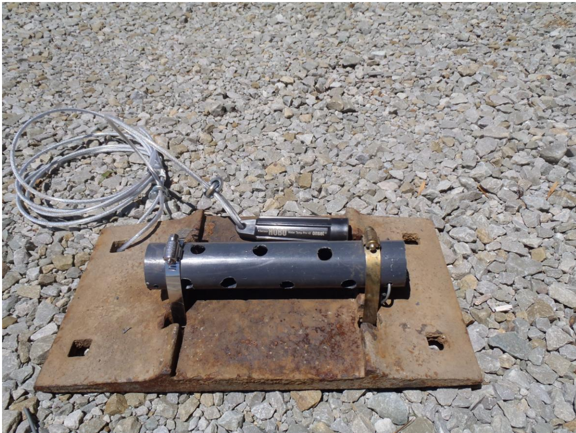
Figure 51. Above, a HOBO water temperature logger is shown attached to PVC housing.
