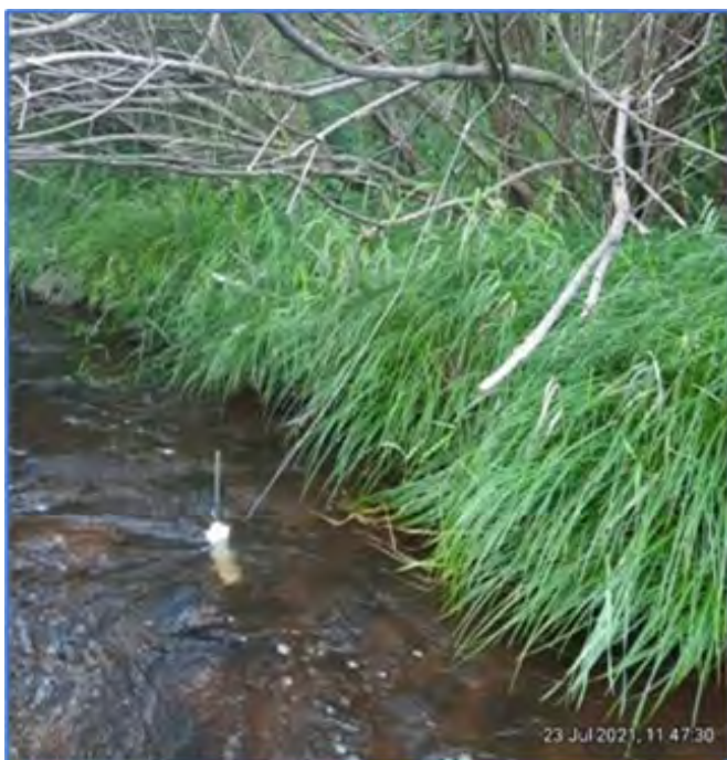
Figure 13 Temperature logger housing deployed on tributary 32264
