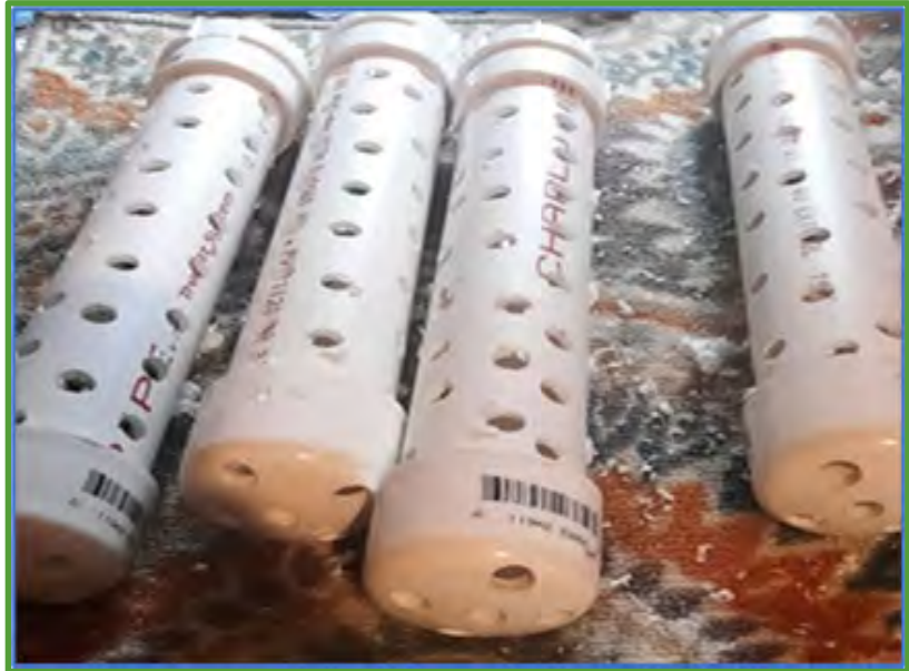
Figure 14 PVC housings for temperature loggers
